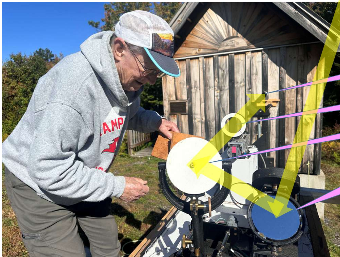
Figure 2: View looking north of the coelostat and objective (foreground) and the SHS building which houses the rest of the instrument (background).
